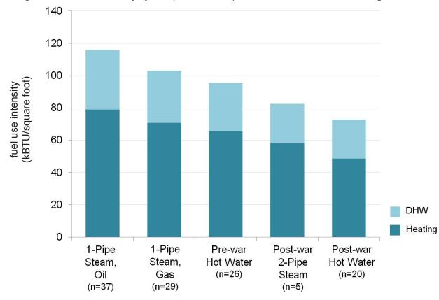
The amount of fuel use dedicated to DHW versus heating was consistent across comparative groups, with about a third of pre-retrofit fuel used for DHW.
