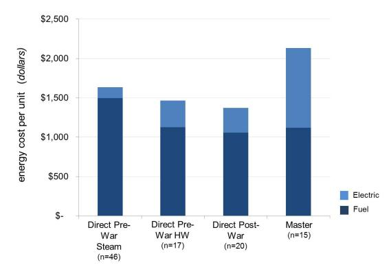
In direct-metered buildings, fuel costs are significantly greater per unit than electric costs.
