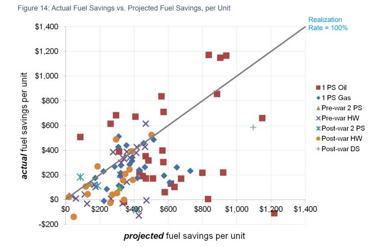
Fuel savings projections tended to range from 25% to 50%, but fuel measures typically resulted in 10% to 40% in savings. Figure 15 indicates projected savings on the Y axis versus project size by unit count on the X axis. Figure 16 indicates actual savings on the Y axis versus project size by unit count on the X axis.
