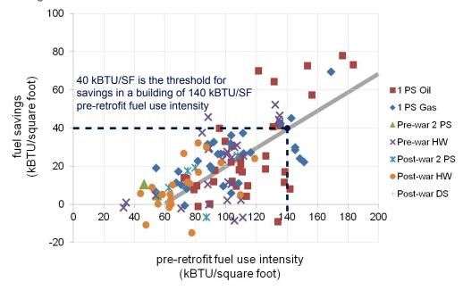
STEP 2: Audit projections are compared to the established threshold. The team reviewed a dataset of 100 projects that had undertaken fuel measures with comprehensive data: savings projections, pre-, and post-retrofit consumption. In this dataset, 86 of 100 fuel projections exceeded the threshold for savings based on their pre-retrofit fuel use intensity profile.
