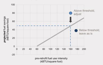
Figure 14: Projected Fuel Savings vs. Actual Fuel Savings, per Unit
