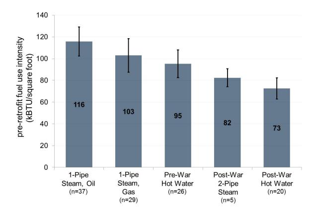
Likewise, each building comparative group tends to have a "retrofit signature," where the scope of a retrofit is significantly a function of the building attributes that define the comparative groups. For instance, a pre-War one-pipe steam building is typically treated by a relatively finite number of energy measures, including controls, distribution upgrades and roof insulation.
